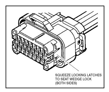
Figure 7-8. Connector Assembly (3 of 4)
