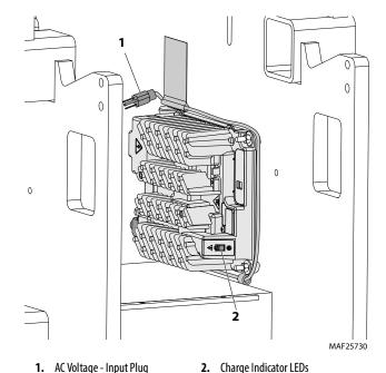
Figure 3-22. Battery Charger (Delta-Q)
