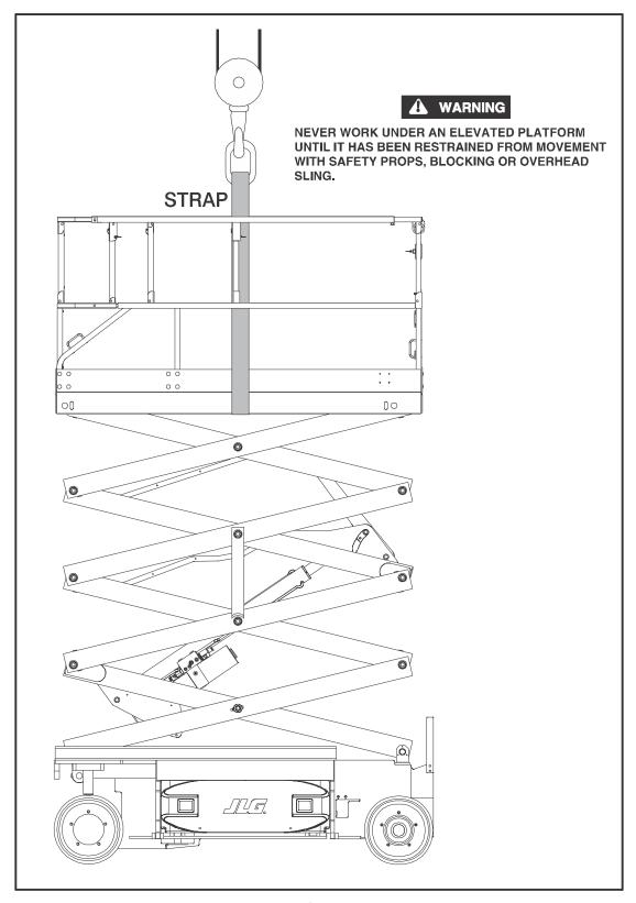
Figure 3-30. Arms and Platform Positioning and Support
