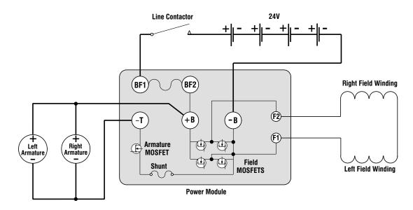
Figure 3-1. Traction Control Circuit - ZAPI Power Module
