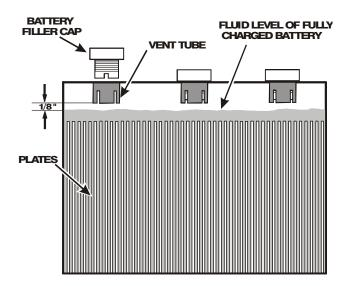
Figure 3-20. Battery Fluid Level
