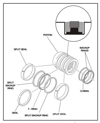
Figure 4-10. Piston Seal Kit Installation
