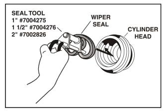
Figure 4-6. Rod Seal Installation
