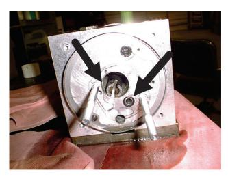
15. Check oring on valve body and replace if necessary before installing the new pump. Lubricate orings before assembling.
