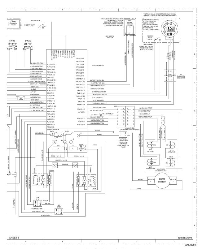
Figure 7-19. Electrical Schematic - Sheet 2 of 10
