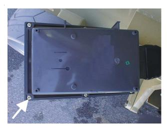
5. Remove the six bolts at the back of the ground control and separate.
