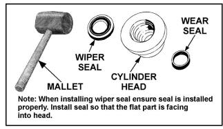
Figure 4-8. Wiper Seal Installation
