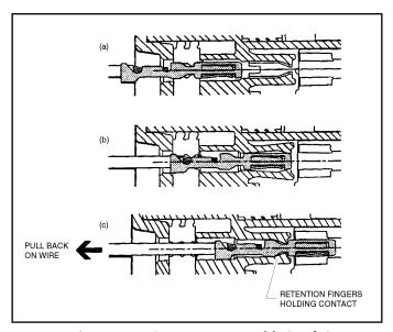
Figure 7-7. Connector Assembly (2 of 4)
