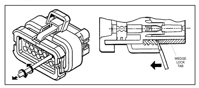
Figure 7-10. Connector Disassembly
