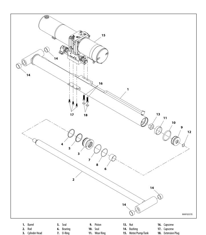
Figure 4-14. Lift Cylinder Assembly (1930ES) (SH-PAC)
