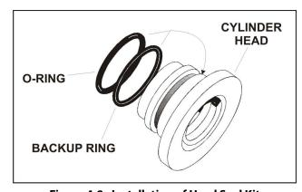
Figure 4-9. Installation of Head Seal Kit
