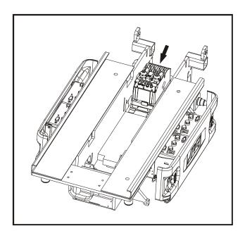
Figure 3-24. Battery Charger/Inverter Location
