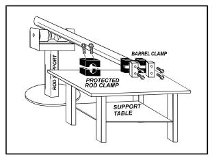
Figure 4-3. Cylinder Barrel Support
