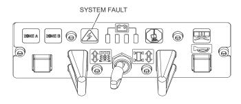
Diagnostic Trouble Codes are indicated on the MDI for those machines that are equipped with an MDI. (refer to Section 3.7).
