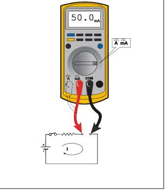
Figure 7-4. Current Measurement (DC)
