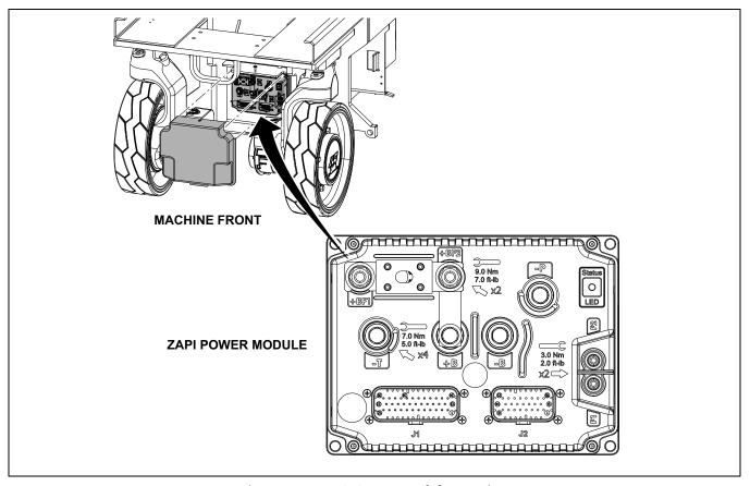
Figure 3-18. ZAPI Power Module Location
