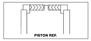
Figure 4-7. Poly-Pak Piston Seal Installation
