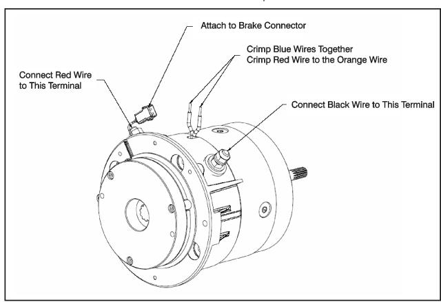
Figure 3-17. Wire Harness Connections
