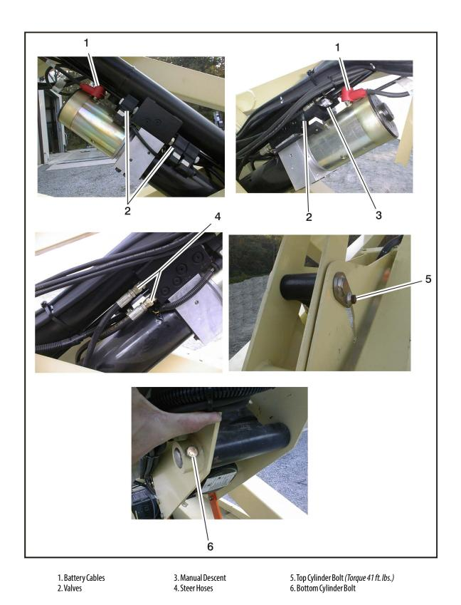
Figure 4-2. LIft Cylinder Removal
