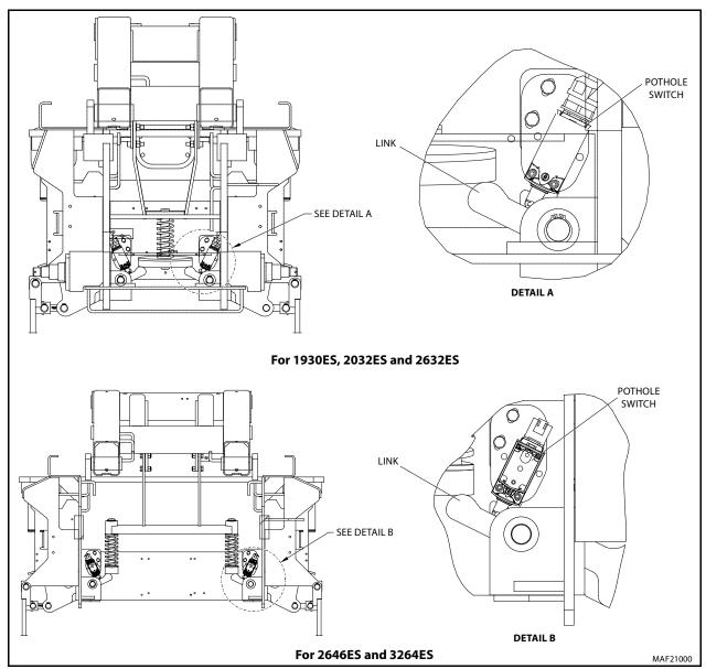
Figure 3-27. Pothole Switch Adjustment
