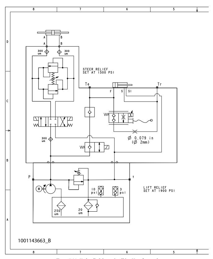
Figure 7-30. Hydraulic Schematic - China Manufactured
