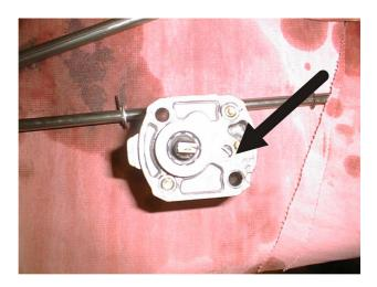
**NOTE:** Be sure to remove and discard the plastic plug at the oil inlet on the new pump before installing.
