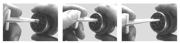
Figure 7-16. HD/HDP Contact Removal
