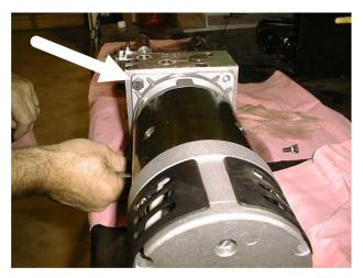
Remove the four bolts attaching the motor to the valve body.
