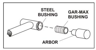
Figure 4-5. Gar-Max Bearing Installation
