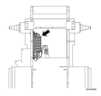
Figure 3-21. Battery Charger Location
