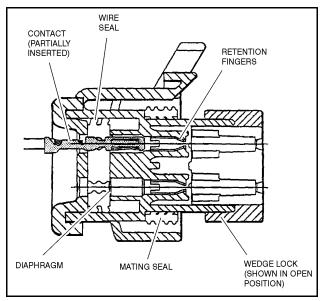
Figure 7-6. Connector Assembly (1 of 4)
