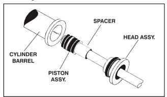
Figure 4-11. Rod Assembly Installation
