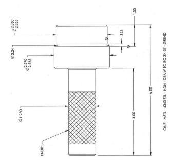
Figure 3-13. Assembly Tool 2
