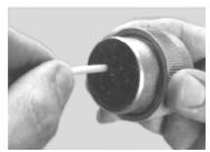
Figure 7-14. HD/HDP Contact Installation
