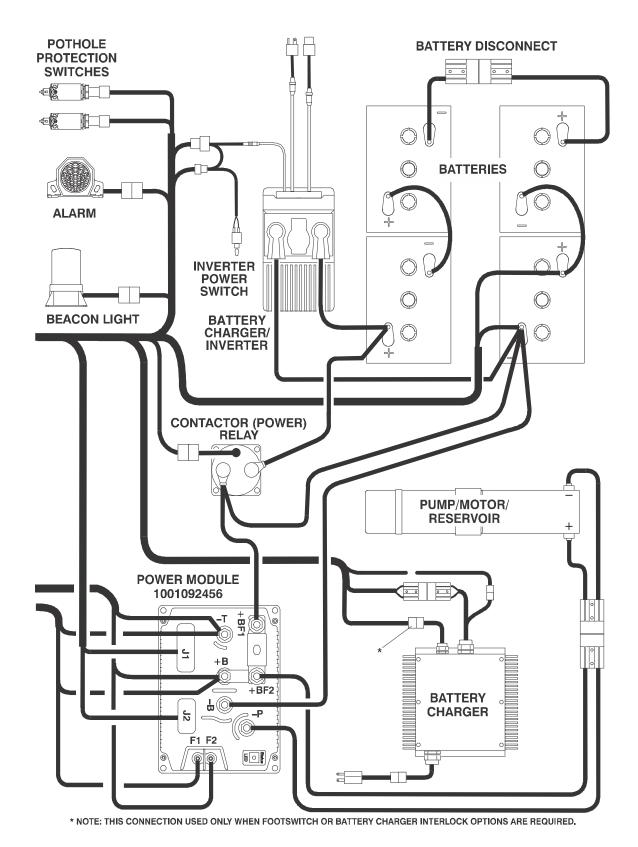
Figure 7-28., Electrical Components Layout
