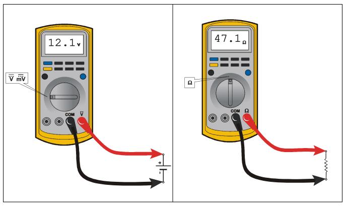
Figure 7-1. Voltage Measurement (DC)
