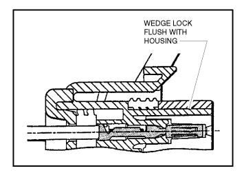
Figure 7-9. Connector Assembly (4 of 4)
