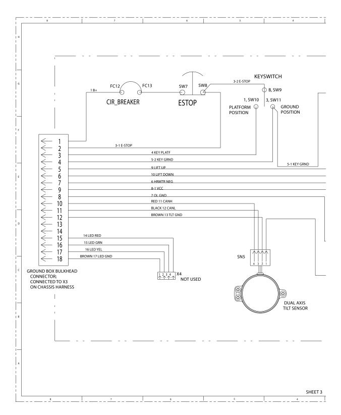
Figure 7-22. Electrical Schematic - Sheet 5 of 10
