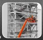
More Capacity With a dual 450/230 kg capacity, the platform can handle more workers, tools or materials.
