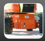
Manoeuvrability Optimum manoeuvrability with 4-wheel steer.
