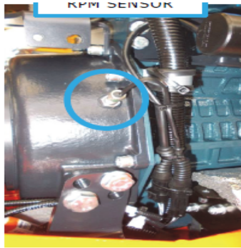
Figure 3-31. Speed Sensor on Kubota D902
