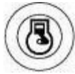
Figure 6-44. Allows the engine to be switched on/off. If the button is pressed with the engine on, this will be stopped.
