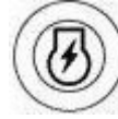
Figure 6-45. Allows the electric motor to be switched on/off. If the button is pressed with the engine on, this will be stopped.
