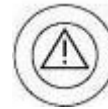
Figure 6-39. Used to enable control of the emergency descent from the basket. Confirmation that the operation is enabled is displayed on the screen in position 8.
