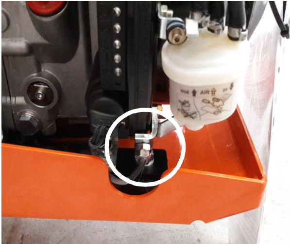
Figure 3-29. Speed Sensor Hatz 1B40
