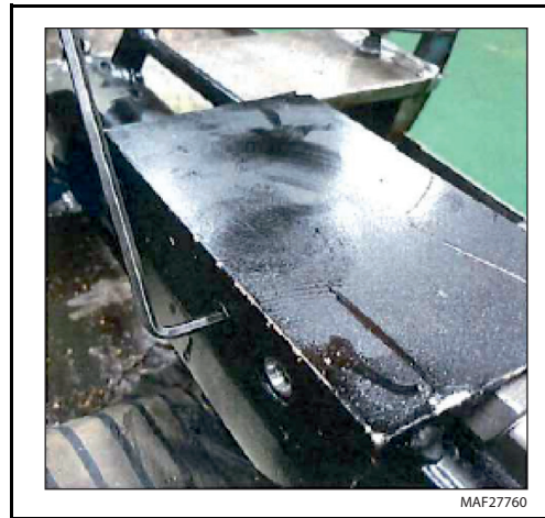
Figure 5-126. Cylinder Plug Removal
