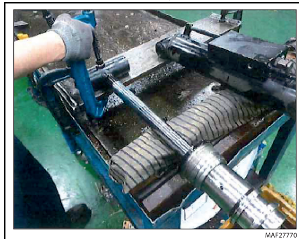
Figure 5-63. Cylinder Rod Support
