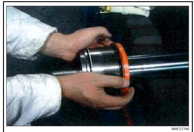
Figure 5-37. Cylinder Head Assembly
