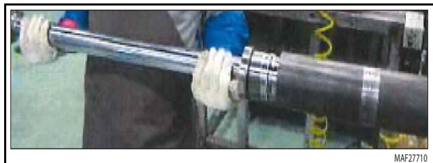
Figure 5-62. Cylinder Rod Removal
