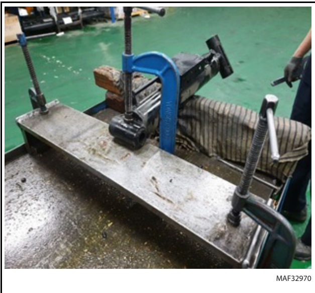
Figure 5-125. Cylinder Clamp Holder
