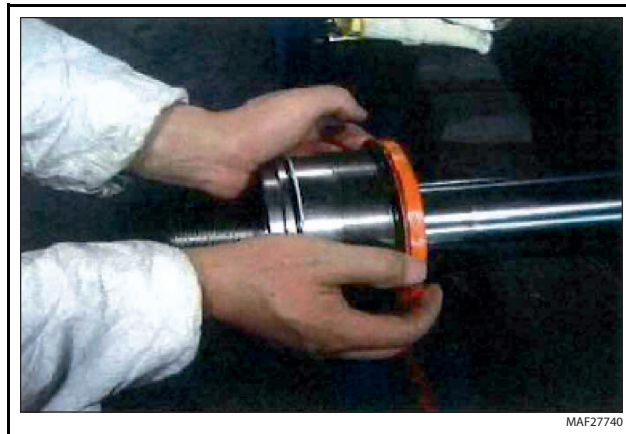
Figure 5-66. Cylinder Head Disassembly
