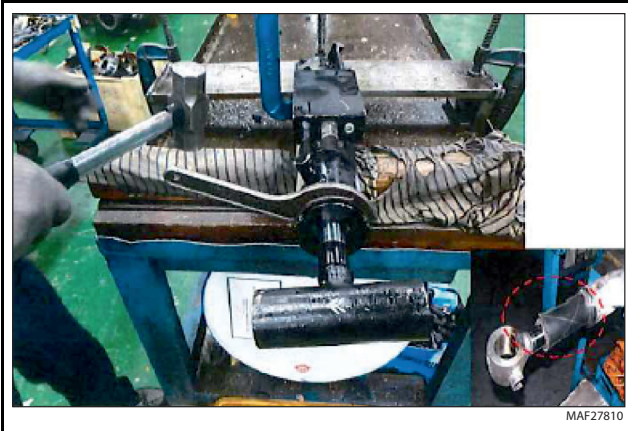
Figure 5-129. Cylinder Head Cover Removal
